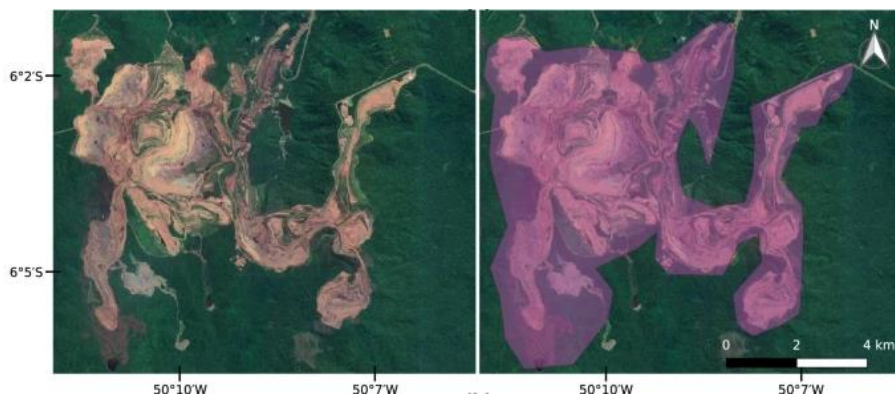
Figure 2: Identifying direct site footprints from aerial photography. Taken from Maus et al 2020 7 . Polygon are drawn around physical footprints to estimate area covered.
