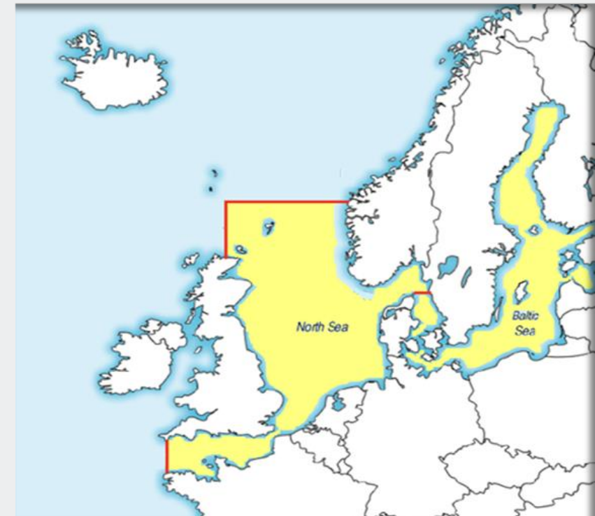
North Sea and Baltic Sea ECAs SO x ; NO x (from 1 January 2021)
