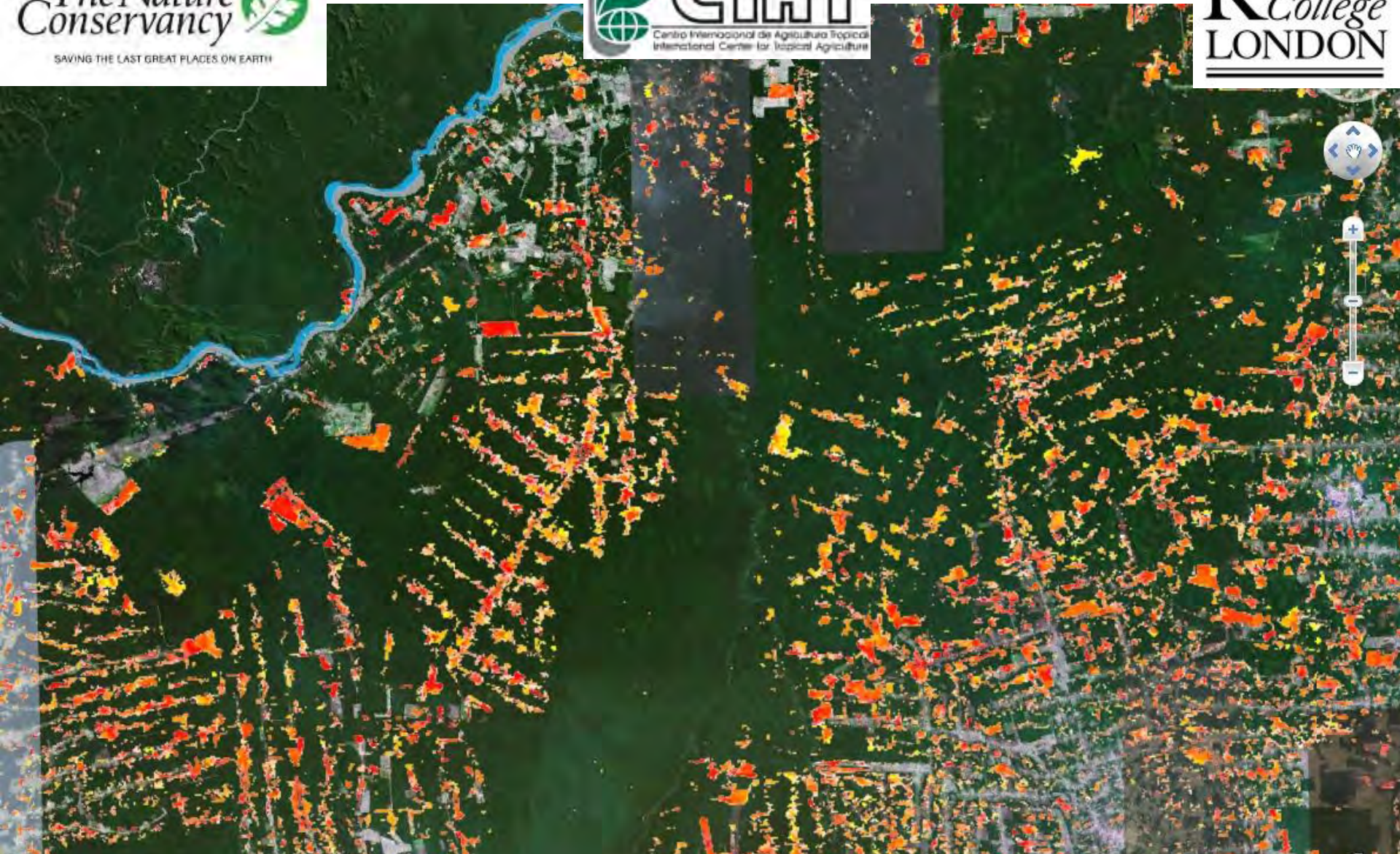
PARASID – dynamic, near real-time 16 day monitoring of land cover change based on neural network analysis of MODIS data. Land use change Rondonia 2004-present (more yellow=more recent)
